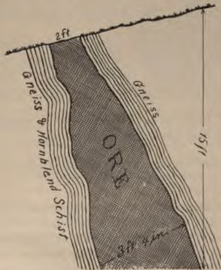
Fig. 47.—Showing ore body at the Blackwell mine, Buncombe county.
